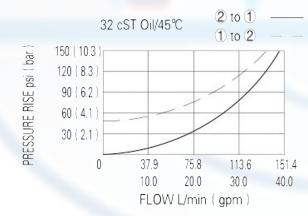
When energized, the valve acts as a check valve, allowing flow from 1 to 2, while blocking flow from 2 to 1;
