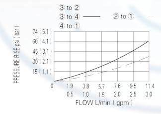
When de-energized, the valve allows flow between the 1, 2, and 4 ports with the 3 port blocked. when the upper solenoid is energized, the valve allows flow between the 2 and 1 parts and the 3 and 4 parts. when the lower solenoid is energized the valve allows flow between the 4 and 1 ports and the 3 and 2 parts.
