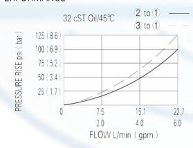
When de-energized, the valve allows flow from 2 to 1, while blocking flow at 3; when energized, the valve allows flow from 3 to 1, while blocking flow at 2.
