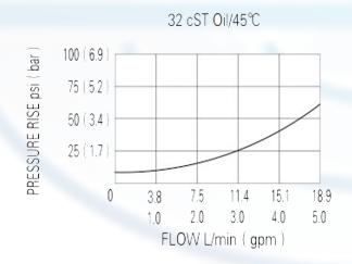
Pressure at 1 overcomes the spring-bias ball and allows free flow 1 to 2.
