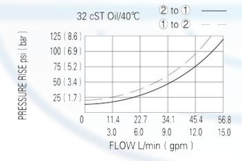
When de-energized, the valve acts as a check valve, allowing flow from 1 to 2, while blocking flow from 2 to 1; when energized, allowing flow from 2 to 1, while 1 to 2 is serverly restrited
