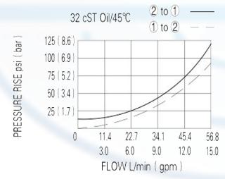
When de-energized, the valve acts as a check valve, allowing flow from 1 to 2, while blocking flow from 2 to 1; when energized, allowing flow from 2 to 1 and 1 to 2
