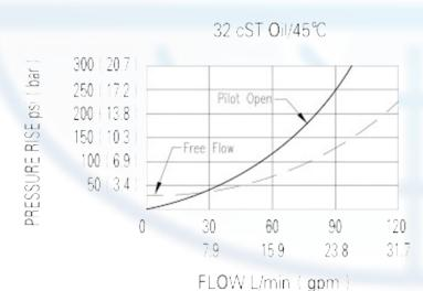
counterbalance valves should be set at leas 1.3 times the maximum load induced pressure.
