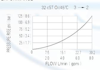
In its steady state, the valve blocks flow from 3 to 2. On attainment of a pre-determined presssure at 1, the cartridge shifts to open at 3 to 2. since the sping, chamber is vented at 2, back pressure at 2 will directly (1:1) affect the valve's setting.
