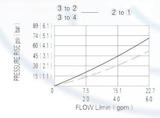
When de-energized, the valve allows flow at all ports.
