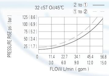
When de-energized, the valve acts as a check valve, allowing flow from 1 to 2, while blocking flow from 2 to 1; when energized, allowing flow from 2 to 1, while 1 to 2 is serverly restrited
