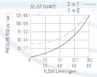
When energized, the valve acts as a check valve, allowing flow from 1 to 2, while blocking flow from 2 to 1;
