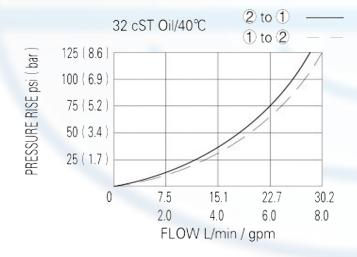
When de-energized, the valve blocks flow in both directionals, when energized, allowing flow from 2 to 1 and 1 to 2
