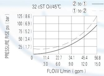
When energized, the valve acts as a check valve, allowing flow from 1 to 2, while blocking flow from 2 to 1; when de-energized, allowing flow from 2 to 1 and 1 to 2
