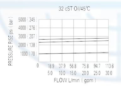
The valve prevents flow from 1 to 2 until pressur at 1 exceeds the set crack pressure and open the pilot section.
