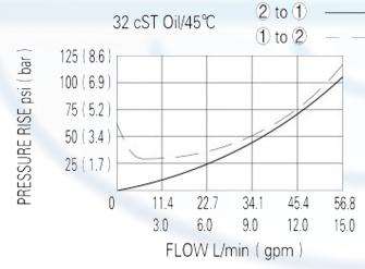
When de-energized, the valve acts as a check valve, allowing flow from 1 to 2, while blocking flow from 2 to 1; when energized, allowing flow from 2 to 1, while 1 to 2 is serverly restricted.
