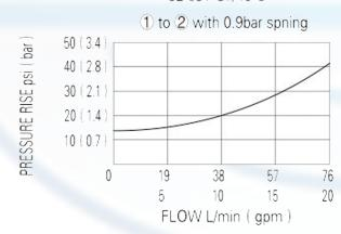
Pressure at 1 overcomes the spring-bias ball and allows free flow 1 to 2.
