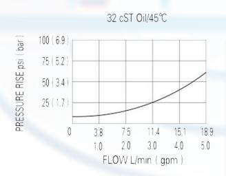
Pressure at 1 overcomes the spring-bias ball and allows free flow 1 to 2.
