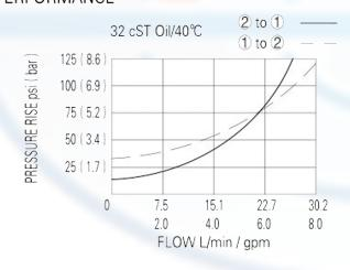
When de-energized, the valve acts as a check valve, allowing flow from 1 to 2, while blocking flow from 2 to 1;
