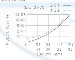
When de-energized, the valve acts as a check valve, allowing flow from 1 to 2, while blocking flow from 2 to 1;
