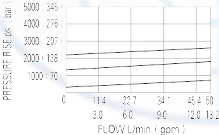
The valve is a direct-acting, dual cross-over relife valve in a single cartridge format. when pressure at either port exceeds the nominal setting value, flow will be transmitted to the opposite port. Back pressure at either port will affect the nominal setting of the opposite port on a 1:1 basis.
