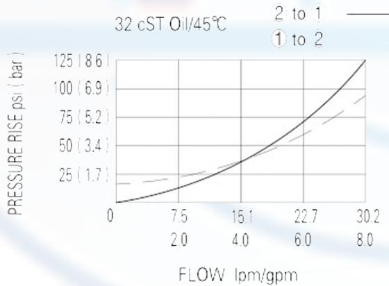
The valve varies flow restriction by adjusting needle in or out. flow is metered from 2 to 1. free reverse flow is from 1 to 2
