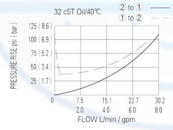
When energized, the valve acts as a check valve, allowing flow from 1 to 2, while blocking flow from 2 to 1;
