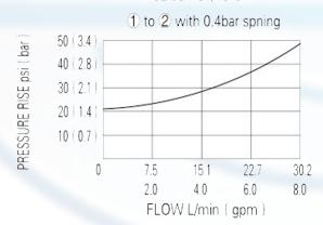
Pressure at 2 overcomes the spring-bias ball and allows free flow 2 to 1.
