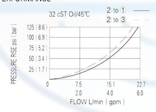
When de-energized, the valve allows flow from 3 to 2, while blocking flow at 1; when energized, the valve allows flow from 2 to 1, while blocking flow at 3.
